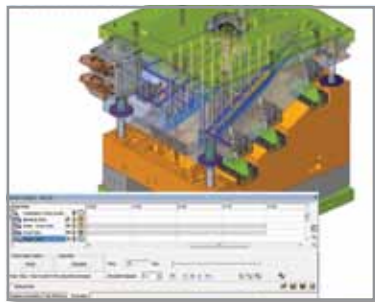
Motion Simulation and Analysis verifies the Kinematics of tool assemblies.
